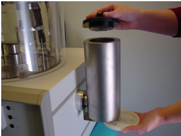
Figure 6: Liquid Nitrogen Cold Trap with Dewar Cap and Drip Trap displayed.
