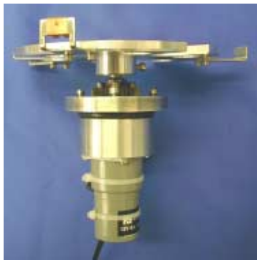
Figure 4-4: Spin Table Shown Mounted Concentrically
