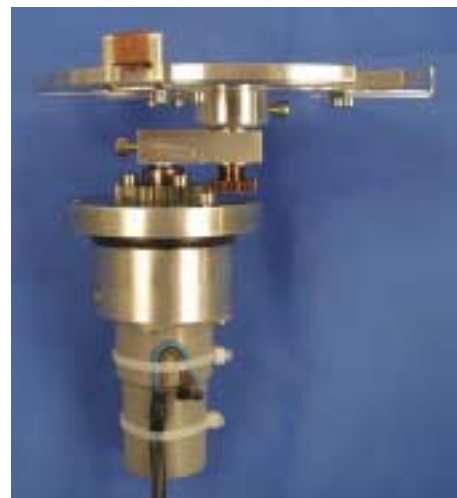
Figure 4-5: Spin Table Shown Mounted Eccentrically
