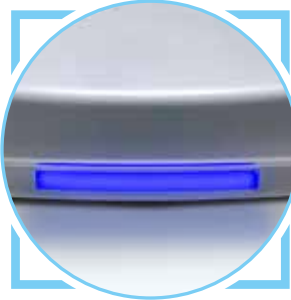
Status indication through multi-colour LED bar
