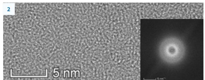
HR TEM image of 10nm carbon layer deposited on 50nm SiN membrane, with a base pressure of  $8E-07$  mbar, and the corresponding FFT.
