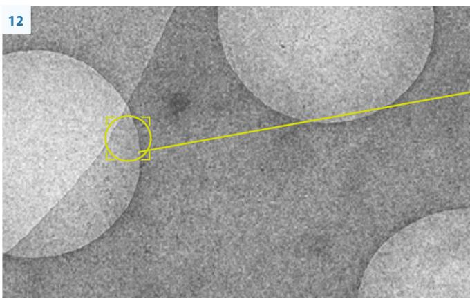
cryo-HR TEM image of DNA replication complex placed onto 200 TEM mesh grid with holey carbon and 5nm additional carbon layer (produced with use of  $8 \times 10^{-7}$  mbar, floated from mica); image showing no flaws of floated carbon film.
