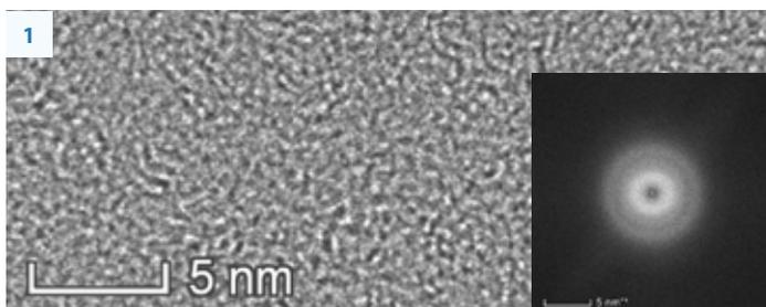
HR TEM image of 10nm carbon layer deposited on 50nm SiN membrane, with a base pressure of  $4E-05$  mbar, and the corresponding FFT.
