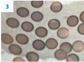
5nm carbon layer produced with base pressure  $4 \times 10^{-5}$  mbar floated from mica onto TEM grid - visible cracks and flaws of the carbon layer.
