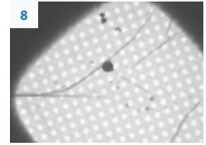
5nm carbon layer produced with base pressure  $8 \times 10^{-7}$  mbar floated from mica onto 200 mesh with holey carbon TEM grids - neat, sturdy and dense layer covering the whole grid.
