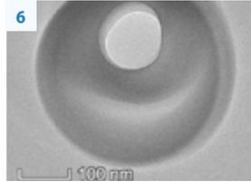
HR TEM image of 5nm C film produced with base pressure  $4 \times 10^{-5}$  mbar, floated from mica onto TEM 200 mesh grid - the amount of hydrocarbons influences the layer stability under the beam, showing visible burn out.
