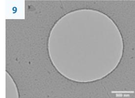
HRTEM image of 5nm C film produced with base pressure  $8 \times 10^{-7}$  mbar, floated from mica onto TEM 200 mesh grid - sturdy and even layer.
