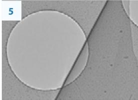
HR TEM image of 5nm C film produced with base pressure  $4 \times 10^{-5}$  mbar, floated from mica onto TEM 200 mesh grid - breaks in the carbon layer and an overlap of the layer caused by poor mechanical stability.
