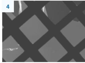
5nm carbon layer produced with base pressure  $4 \times 10^{-5}$  mbar floated from mica onto 200 mesh TEM grids - visible cracks and wrinkles, and the carbon is not covering the whole grid.
