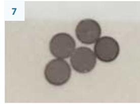
5nm carbon layer produced with base pressure  $8 \times 10^{-7}$  mbar floated from mica onto TEM grids - neat, sturdy and dense layer.
