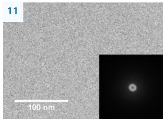
HR TEM image and corresponding FFT of 5nm C film produced with base pressure  $8 \times 10^{-7}$  mbar, floated from mica onto TEM 200 mesh grid showing the film quality.
