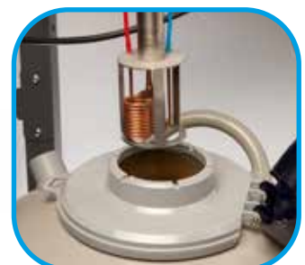
Heat exchanger and dewar
